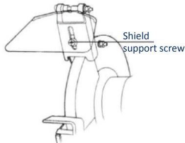
1. Loosen the shield support screw.
