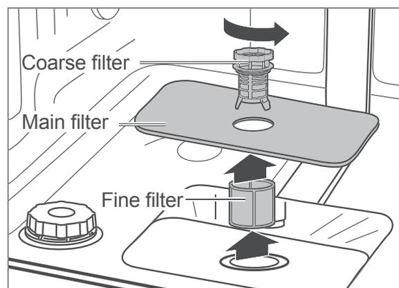
Check the coarse filter, the main filter and the fine filter after each rinse cycle and remove food residues and foreign bodies if necessary.
