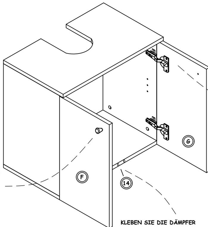
KLEBEN SIE DIE DÄMPFER AUF DIE STIRNKANTE DES UNTEREN BRETTS.
