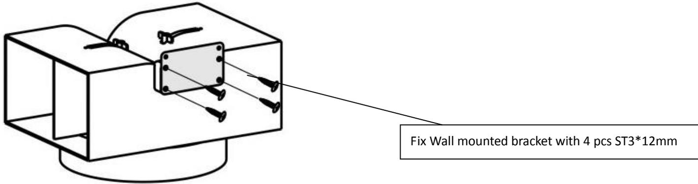
( pls check the length of air diffuser before installation ,if it is enough long to match the width of inner chimney, there is no need to fix the left and right T-shape , if not, pls ajust the length of T-shape and fix them with screws 2pcs ST3\*12mm ).
