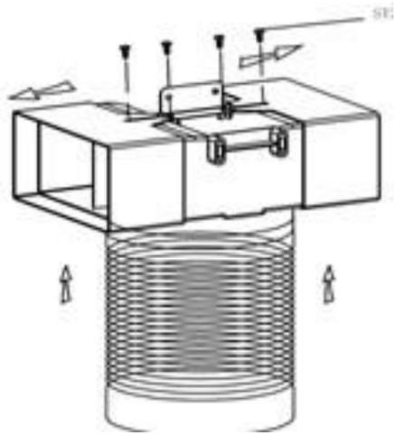
3. Fix hanging bracket A + hanging bracket B together with 2 pcs ST4\*8mm screw, ensure the inner chimney can extensible , You may have to ajust the length of air diffuser, make sure it's available to the width of inner chimney . (Pic.C)
