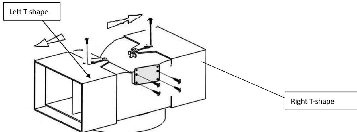
2 . Drill 2 holes with the diameter of 8mm on the wall ,insert the plastic wall plug and Fix above combination with 2 pcs screw ST4\*30mm in it , then connect the extension pipe to the air diffuser(pic B) .
