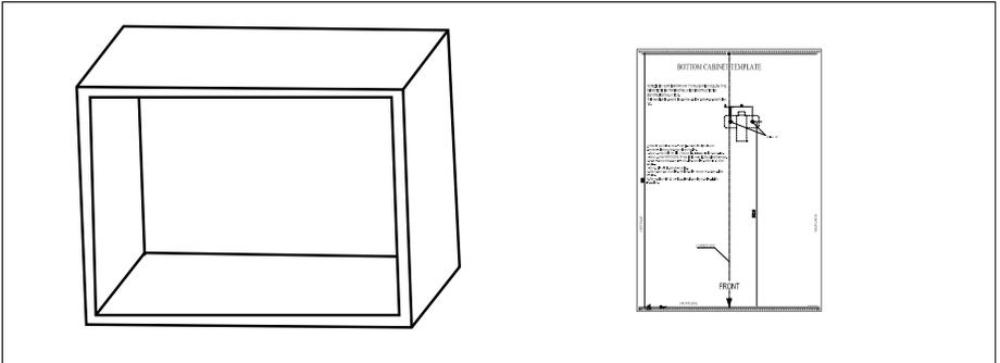
2. Make the marks on the bottom plane of cabinet according to marks "a" of the template.
