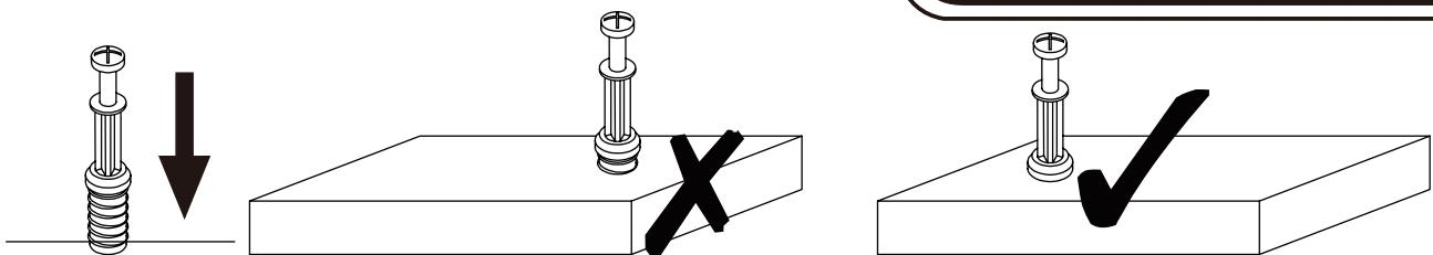
**EN\_QUICKFIT:** Tighten quickfit until shoulder is flush with panel. Do not overtighten or undertighten.
