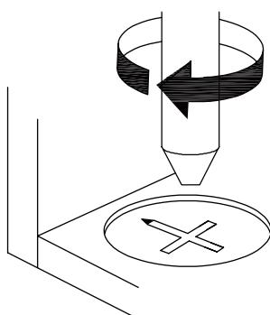
**EN**\_Turn cam lock clockwise to tighten.
