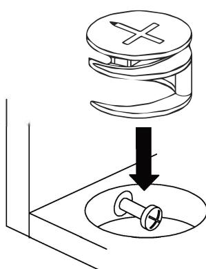
**EN**\_Quickfit head should be in the centre of the cam lock when the two panels are joined.
