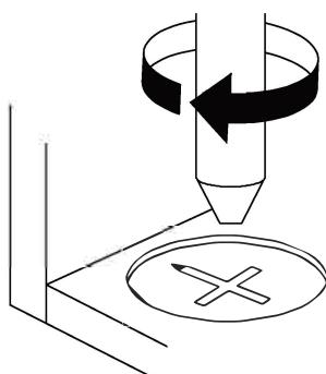
**EN**\_Turn cam lock clockwise to tighten.
