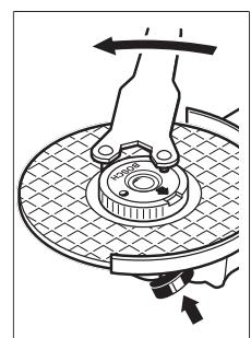
If the quick-clamping nut has been attached correctly and is not damaged, you can loosen it by hand by turning the knurled ring anticlockwise. **If the quick-clamping nut is stuck, do not attempt to loosen it with pliers – always use the two-pin spanner.** Position the two-pin spanner as shown in the figure.
