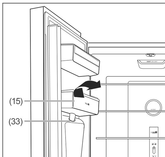
1. Remove the water tank (15) from the holder (33).
