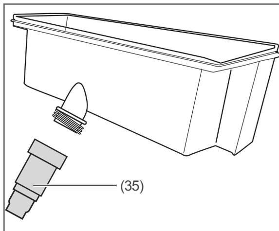
5. Unscrew the outlet valve (35) from the water tank and then disassemble the valve.
