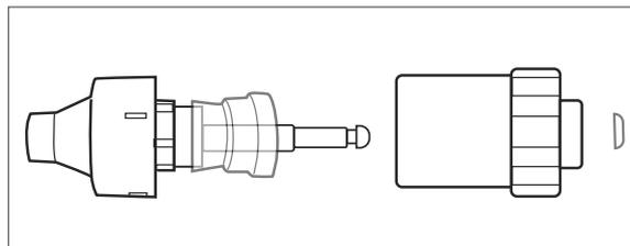
6. Wash the individual parts of the outlet valve likewise with warm, soapy water and then rinse them well with clean water.
