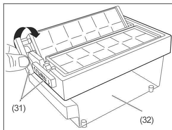
2. To remove ice cubes, turn the levers (31) clockwise.
