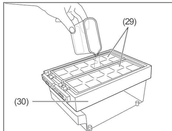
1. Fill the ice cube moulds (29) of the included ice maker (30) to approx.  $\frac{3}{4}$  full with fresh drinking water and place the ice maker horizontally in the freezer. You should ideally use a jug (not included) to do this.
