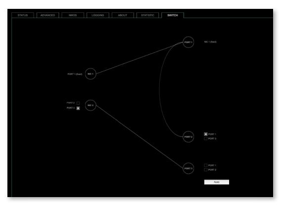
Two independent network interfaces (NICs) can be configured in the switch configuration.
