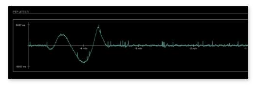
Graphical display of measured PTP jitter.
