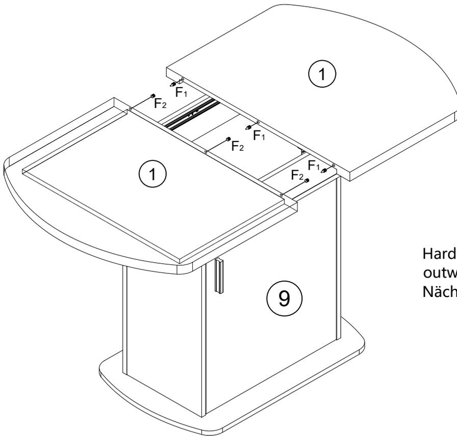
Hardware F2 has a hole at one end facing outward
