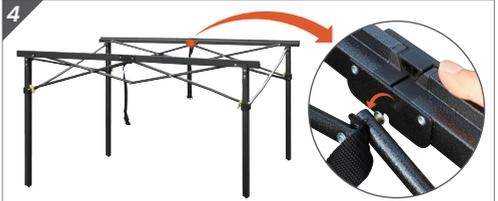
4 Identify the notches in the frame beams and the protruding rivets in the cross bracing tubes. Align the notch in the middle of the frame beam with the protruding rivet on the cross tube and snap it in.
