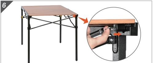
6 Locate the latch on the underside of the table corner, insert the latch lock into the corresponding lock hole on the frame.
