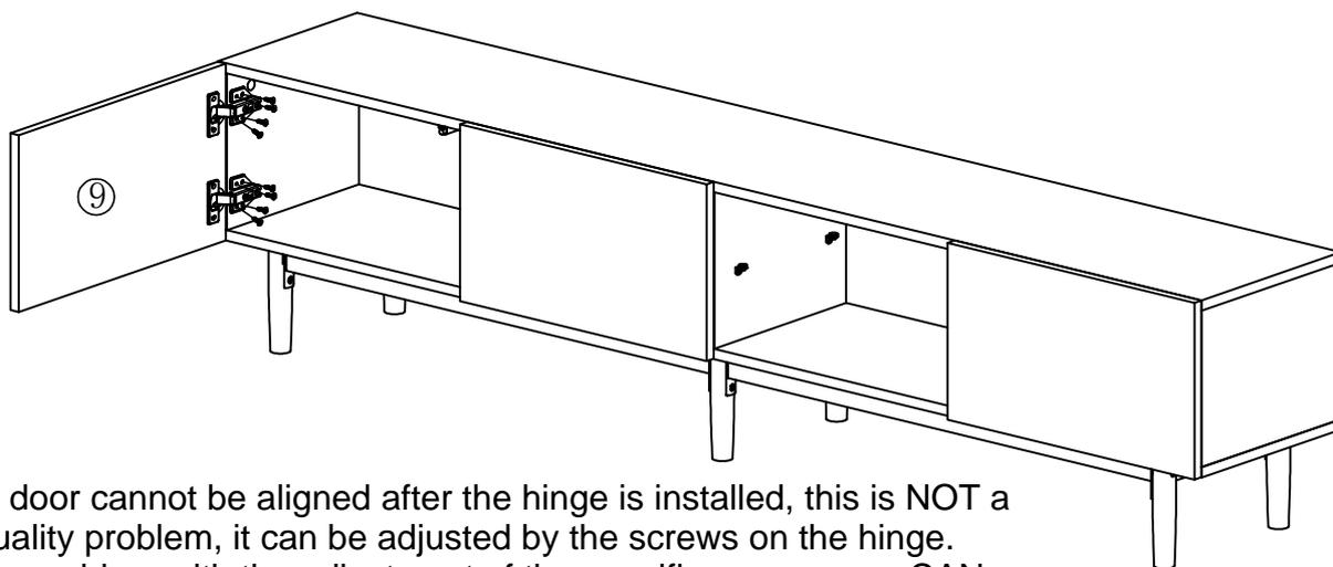
Tips: If the door cannot be aligned after the hinge is installed, this is NOT a product quality problem, it can be adjusted by the screws on the hinge. If there is a problem with the adjustment of the specific screws, you CAN CONTACT the service provider to obtain an adjustment plan.
