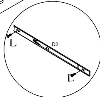
If the drawer is skewed, please remove the drawer and check whether the screws fixing the slide rails are installed on the same horizontal or vertical line. If they are not on the same horizontal line, please readjust the installation.
