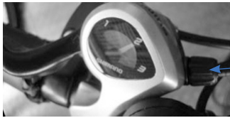
Knurled nut for fine adjustment
