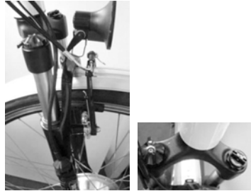
Adjustable suspension forks with lock-out and adjustment
