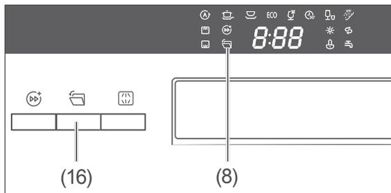
The “Automatic door opening” function is activated as standard. The appliance door opens automatically during the drying phase of the dishwashing programme and remains open. This ensures particularly efficient drying. Wait for the programme to end before removing the dishes to achieve the best possible drying result.
