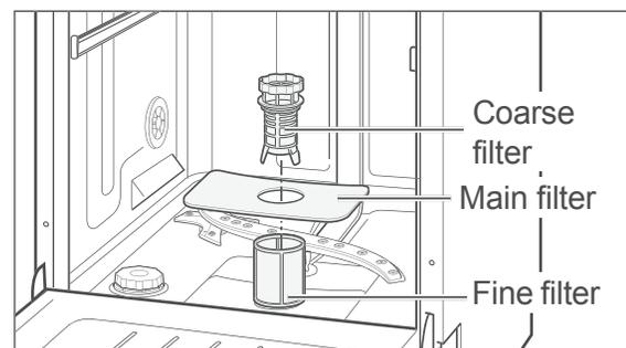
Check the coarse filter, the main filter and the fine filter after each rinse cycle and remove food residues and foreign bodies if necessary:
