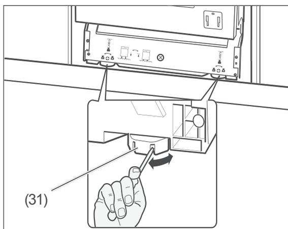
8. To position the dishwasher so that it is level, the two front adjustable feet (31) and the back foot on the appliance can be adjusted by up to 50 mm.
