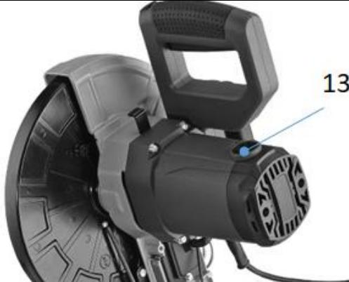
Check the carbon brushes after the first 50 hours of operation with a new machine or when new brushes are installed. After performing the first check, repeat the check every 10 operating hours.
