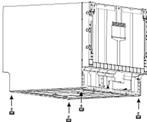
3. Insert the appliance into the installation opening carefully. Align the supporting feet on the bottom of the installation opening (**A** / s. fig. below).
