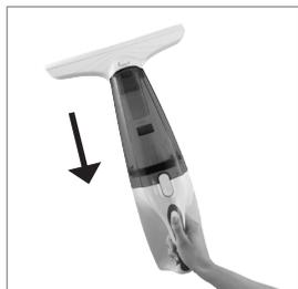
3. Guide the nozzle (4) over the surface to be cleaned from top to bottom. During use, check whether the collecting container (5) is full. If this is the case, it needs to be emptied.
