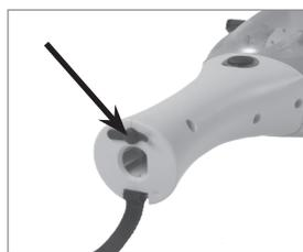
1. Connect the barrel connector of the mains adapter (7) to the main unit.
