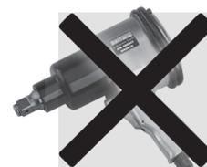
The force screw maximum recommended torque is 170Nm (M18x1.5), 155Nm (M16X1.5), 99Nm (M14X1.5), 60Nm (M12X1.5), 33Nm (M10X1.5).
