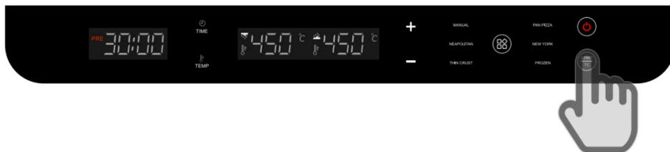
7. During the preheating process, the PRE indicator on the clock display starts calculating time and the preheat indicator lights up, e.g. 00:01...00:02...00:03. When the temperature reaches the preset temperature, the preheat clock indicator goes out and the display changes to the pizza countdown time. There will also be a beep to prompt you to put the pizza in.
