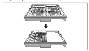
To remove the right-hand cutlery grid, lift the cutlery grid on the left side, move the left pair of rollers through the guide groove past the stopper and slide the cutlery grid all the way to the left.
