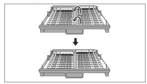
To straighten the right-hand cutlery grid, lift the cutlery grid on the left side and move the left pair of rollers through the guide groove past the stopper.
