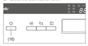
3. If the dishwasher is switched on, switch it off with the  $\circ$  button (18).
