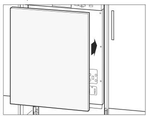
16. Attach the front panel to the appliance door of the dishwasher using the hookand-loop straps (40), hold the panel in place, and carefully open the appliance door.
