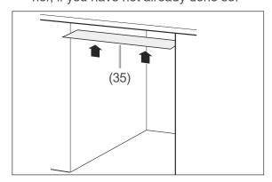
3. Affix the enclosed protective film (35) to the bottom of the worktop. In this way, you will avoid damage to the worktop caused
