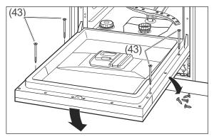
17. Remove the 4 screws from the inside of the appliance door. Screw the front panel in place at these positions using the 4 enclosed screws (43).
