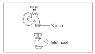
For water supply, you need a water tap with a 3/4-inch screw connector.
