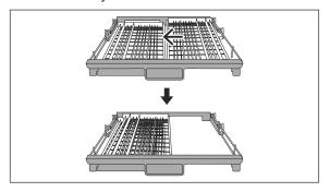
To remove the right-hand cutlery grid, lift the cutlery grid on the left side, move the left pair of rollers through the guide groove past the stopper, slide the cutlery grid all the way to the left and lift it up.
