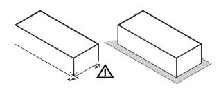
IT IS RECOMMENDED THAT THE ANTI-TIP KIT INCLUDED WITH THIS PRODUCT BE INSTALLED FOR ADDED SAFETY AND STABILITY.
