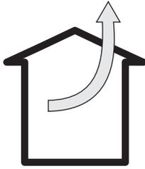
In the extractor mode air is discharged to the outside by a special conduit. In that setting any charcoal filters shall be removed.
