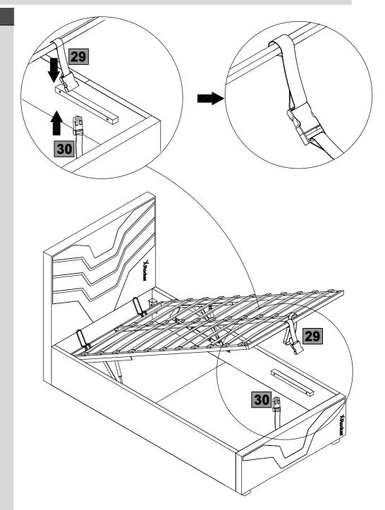
Warning: Lock the buckle after close of gas-lift to avoid opening automatically
