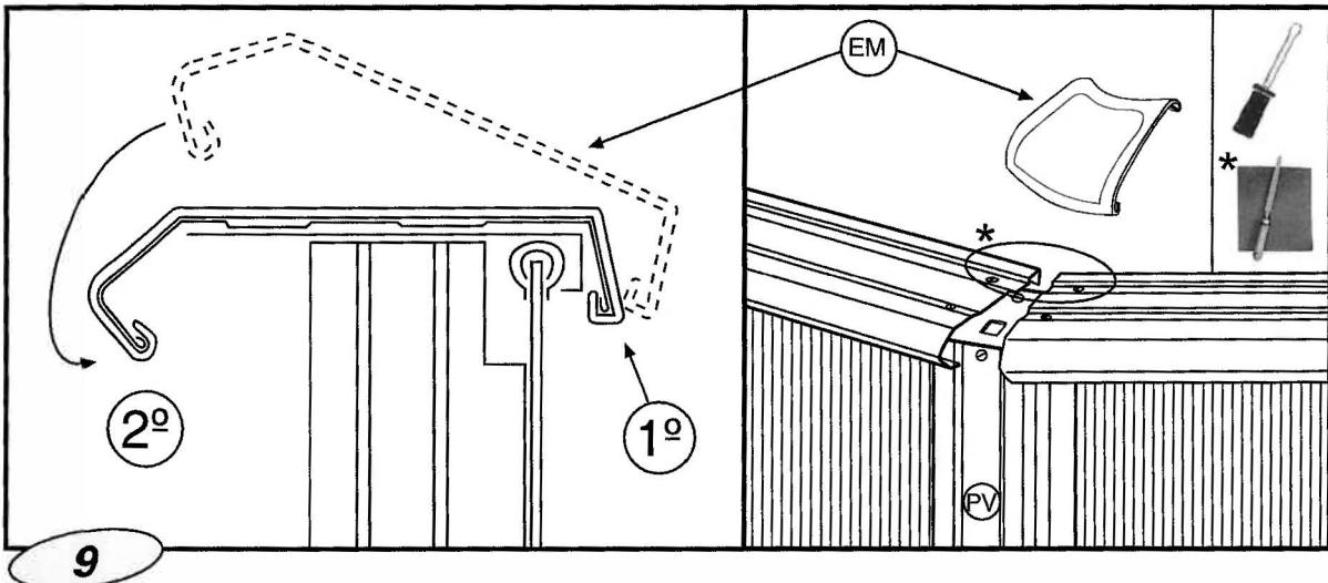
**EN** \* **IMPORTANT! BEFORE ASSEMBLY, DEBURRING, USING A FILE AND SANDPAPER, THE ENDS OF EACH EDGE.**
