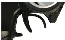
2. Slowly pull the throttle/brake lever towards the handle to make the vehicle move forwards.
