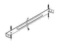
2. Align, mark and drill holes to apply the screws
