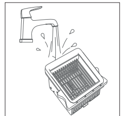
Fig. 18 – Cleaning the filter
