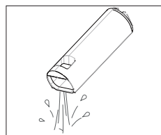
Fig. 10 – Emptying the water tank
