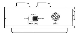
**Low Cut**: a variable high-pass filter, labeled **low cut**, can be used to remove sub-sonic frequencies present in some passive pickups.
