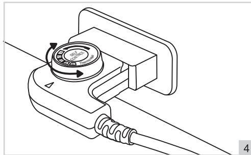
5. After a few minutes the indicator light will go out. Once the indicator light has extinguished the appliance has reached the required temperature, and is ready for use.
