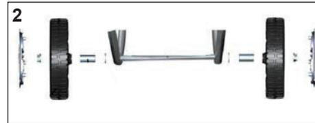
Place the supplied threaded spacer on the axle. Then attach the wheels and finally the safety nuts with the wheel covers.
