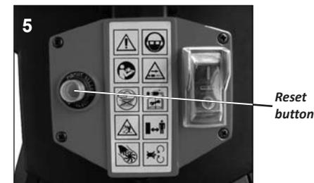
Wait at least 1 minute before restarting by first pressing the reset button and then the on/off switch. If the motor does not start, proceed as follows:
