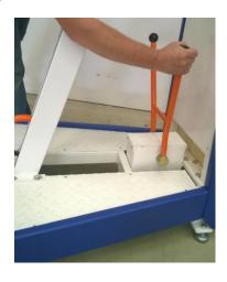
3. Now that the SAM School is in the right place, it needs to be attached to the floor. Attach a carabiner to the D-lock and secure it to a floor hook. By turning the star nob clockwise, turn the toggle screw upwards and tighten the whole.
