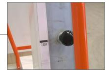
5. Storage: Pull out the catch and pull the mast down to the lowest position using the bracket. The catch gets into the hole and the mast is locked.
