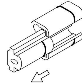
You can pull the buckle out by following the direction indicated by the arrow
