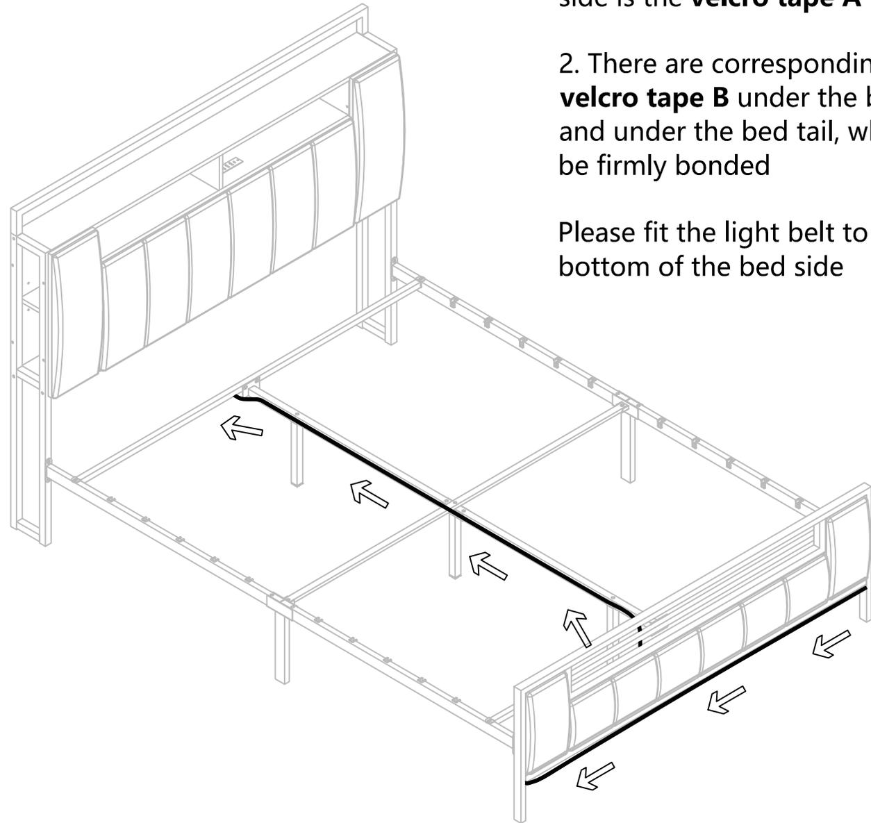
1. One side of the light bar is the luminous surface, and the other side is the **velcro tape A**
