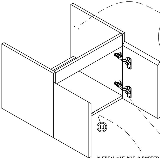
KLEBEN SIE DIE DÄMPFER AUF DIE STIRNKANTE DES UNTEREN BRETTS.
