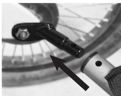
POUSSÉZ LE RACCORD ROND DU TIMON SUR LA PIÈCE D'ATTELAGE MONTÉE SUR LE VÉLO AUSSI LOIN QUE POSSIBLE.
