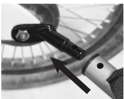
PUSH THE ROUND DRAWBAR CONNECTION OVER THE COUPLING UNIT ATTACHED TO THE BICYCLE.
