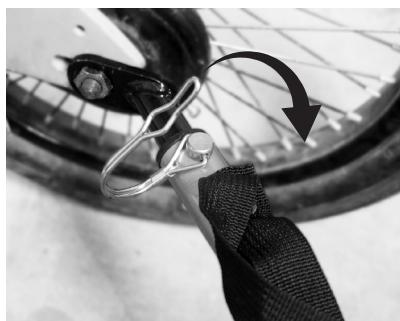
INSERT THE SPRING CLIP BOLT THROUGH THE BOREHOLES OF BOTH COUPLING PARTS AND CLOSE THE CLIP SO THAT THE CLIP OPENING SURROUNDS THE BOLT END.
