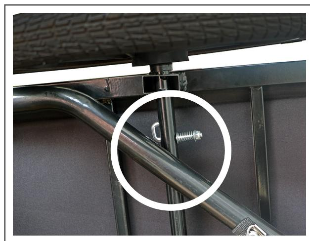
INSERT THE SECURING PIN THROUGH THE HOLE IN THE AXLE AND TIGHTEN IT.
