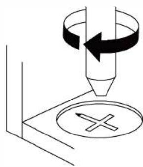
**EN**\_Turn cam lock clockwise to tighten.
