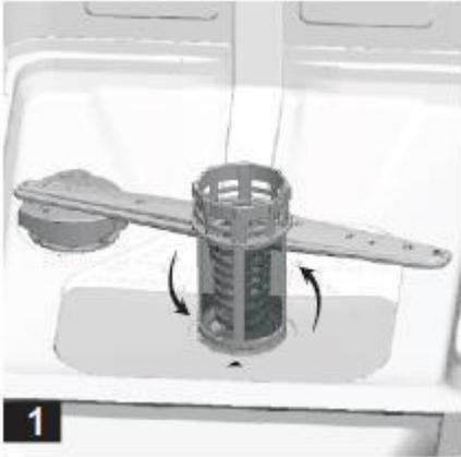
A black and white photograph showing the interior of a washing machine. A central agitator is visible. A cylindrical coarse filter is being turned anticlockwise, as indicated by curved arrows. A small black box with the number '1' is in the bottom left corner of the image.                                 |
