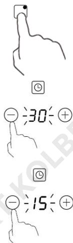
5. When the time is set, the timer starts automatically. The timer display will stop flashing and indicate the remaining time.
