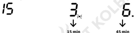
2. As soon as the countdown has expired, the corresponding zone is switched off. The display jumps to the next programmed cooking zone.
