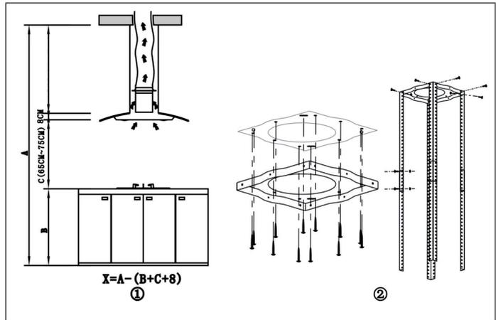
3. Pass one end of the exhaust hose through the hole in the ceiling (see Figure 3).
