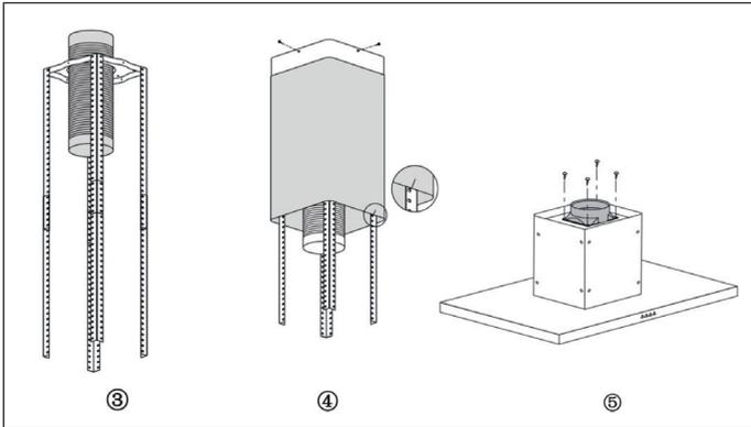
6. Hold the exhaust hood up and fasten it with 16 M4\*10 screws (see Fig. 6).
