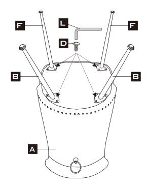
Note: Put all the screws into the hole site, And then tighten them. Donot tighten one by one
