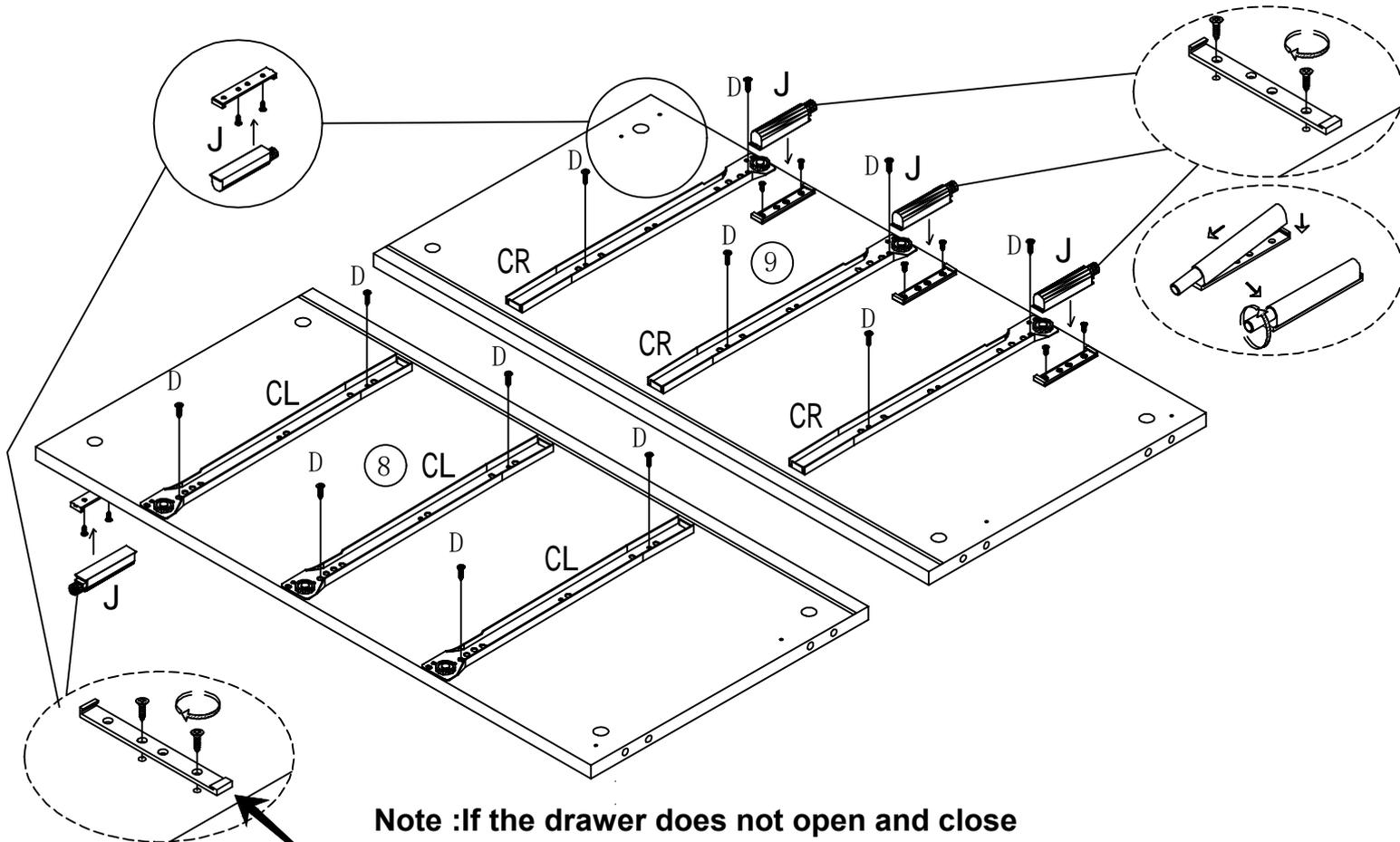
**Note :** If the drawer does not open and close smoothly, you can rotate and adjust this part.
