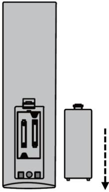
**TV remote control:** Open the battery compartment on the back of the remote control by sliding the cover off the remote control in the direction of the arrow.
