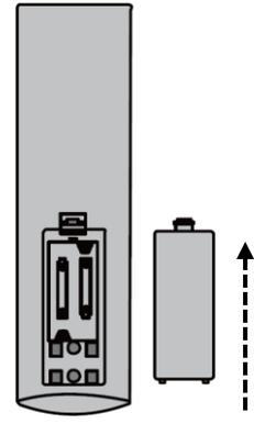
**TV remote control:** Close the battery compartment on the back of the remote control by sliding the cover onto the remote control in the direction of the arrow.
