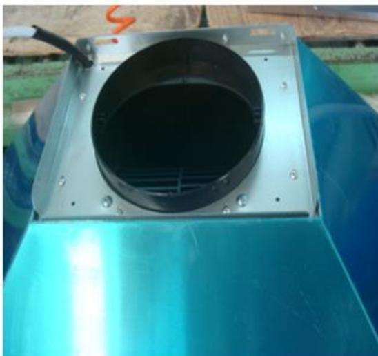
PREASSEMBLED AIR OUTLET FOR FIXING THE EXHAUST HOSE.
