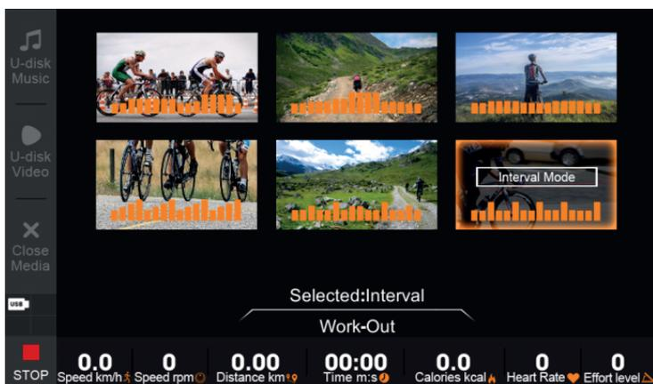
Turn the rotating button to select the desired program and confirm the selection by pressing the rotating button
