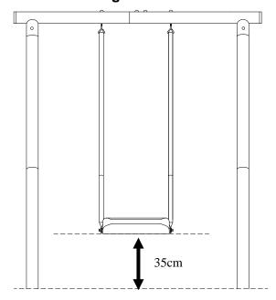
The height of the fully assembled product is 180cm. The minimum ground clearance between the bottom of the suspended swing and the ground surface must be 35cm.
