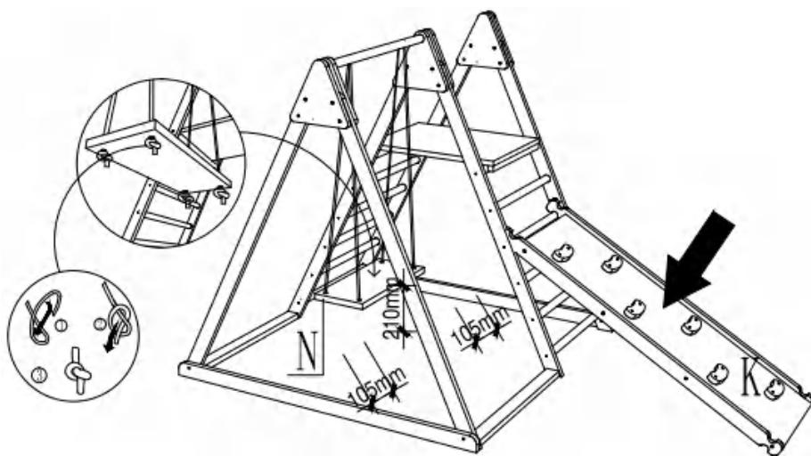
Install the swing into Corresponding position. and place the slide on the first or second round stick of the main body, and the whole installation procedure is complete (**please do not place it on the third or upper round stick, otherwise it will cause danger due to the excessive inclination angle**)
