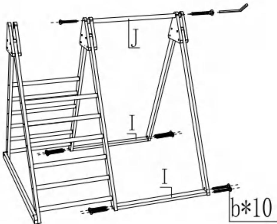
Connect the parts installed in the 3 and 4 steps with 10 pieces of M6\*30.
