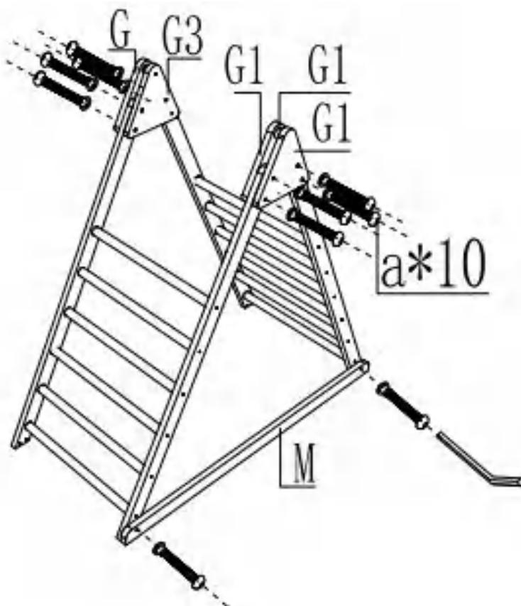
Connect the parts installed in the first and second steps with G, G1, G3, then put the matching decorative block with G1 between the two G1 triangular plate and fix them with 10 pieces of M5\*60. Then, fix the bottom bracket M with 2 pieces of M5\*60 at the bottom of the triangle. Then put it aside for later use.
