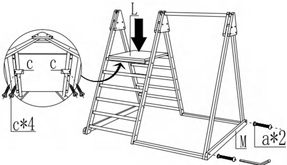
Install the L board on the climbing ladder, and add the M bottom bracket to the bottom of the tripod as shown in the figure, and connect them with two pieces of M6\*30.
