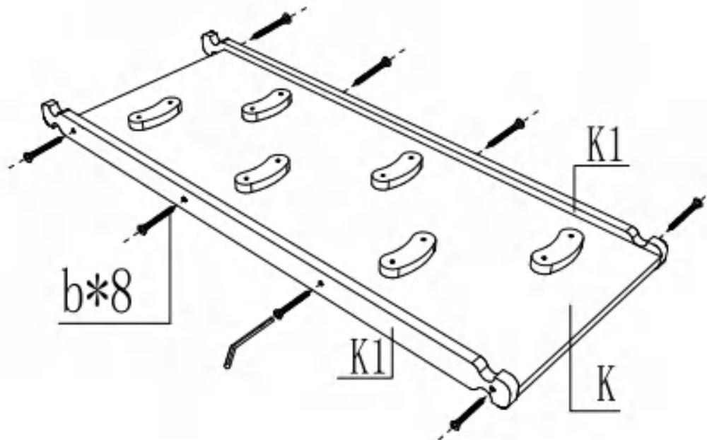
Connect two slide side panels K1 to slide K with 8 M5\*60.
