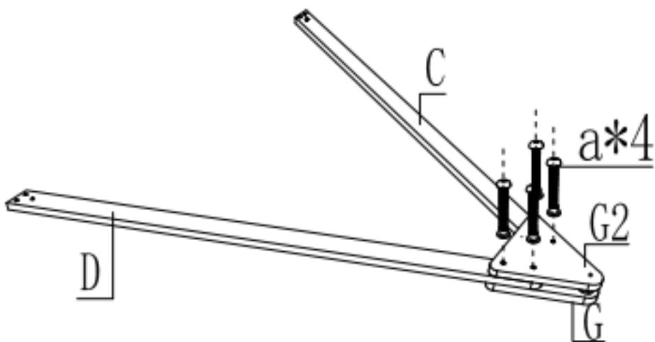
Connect C and D through G and G2 and fix them with 4 pieces of M5\*60. Then put it aside for later use.
