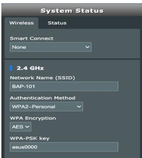
The screenshot shows the 'System Status' screen with the 'Wireless' tab selected. Under 'Smart Connect', the 'None' option is chosen. The '2.4 GHz' section is expanded, showing the following settings: Network Name (SSID) is 'BAP-101', Authentication Method is 'WPA2-Personal', WPA Encryption is 'AES', and WPA-PSK key is 'asus0000'.
