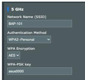
The screenshot shows the 'System Status' screen with the 'Wireless' tab selected. The '5 GHz' section is expanded, showing the following settings: Network Name (SSID) is 'BAP-101', Authentication Method is 'WPA2-Personal', WPA Encryption is 'AES', and WPA-PSK key is 'asus0000'.
