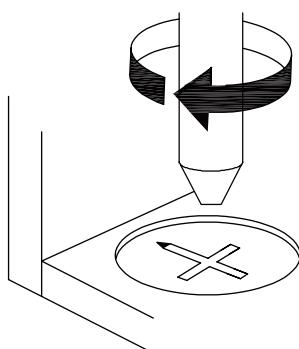
**EN**\_Turn cam lock clockwise to tighten.
