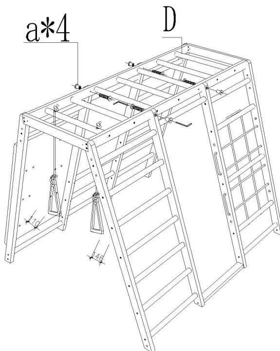
Connect the top of part D and with the climbing frame installed in step 6 and step 7 through 4 pieces of M6\*35 screws.
