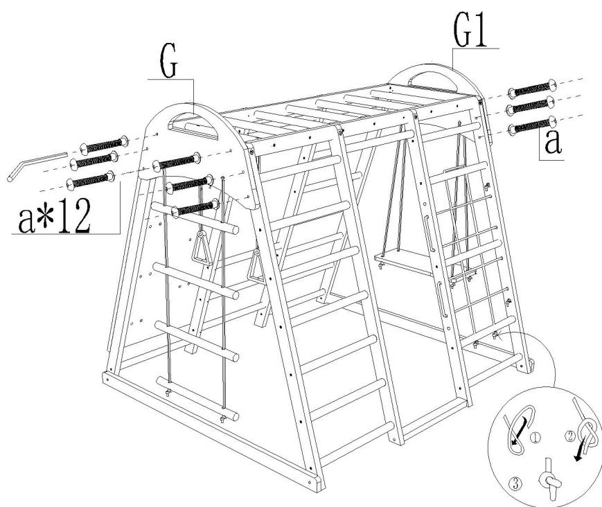
Install the G and G1 with climbing ladder and swing to the side of the climbing frame with 12 pieces of M6\*35 screws.
