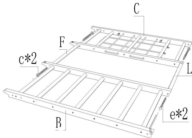
Connect 2 F round sticks between part B and part C, and use 2 pieces of M5\*30 und 2pieces of M3.5\*60 to tighten. Keep it aside for later use.
