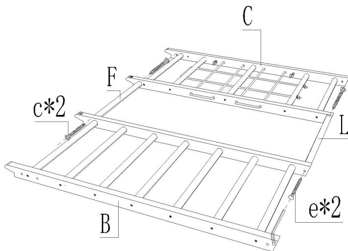
Connect 2 F round sticks between part B and part C, and use 2 pieces of M5\*35 and 2 pieces of M3.5\*60 to tighten. Keep it aside for later use.
