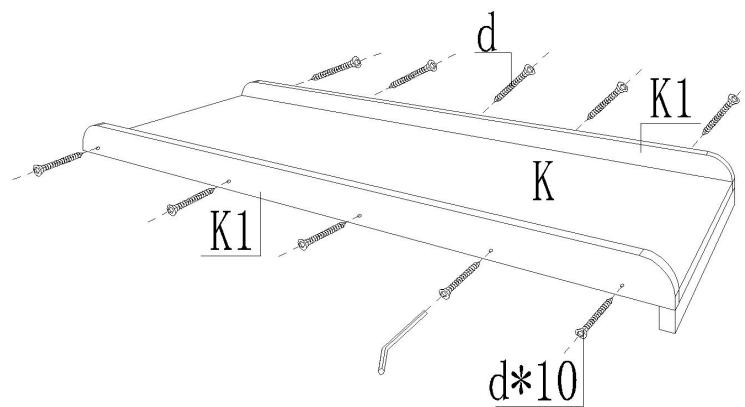
Connect the two slide side panels K1 to the slide K, and fix them with 10 pieces of M5\*35 screws. Set aside for further installation.
