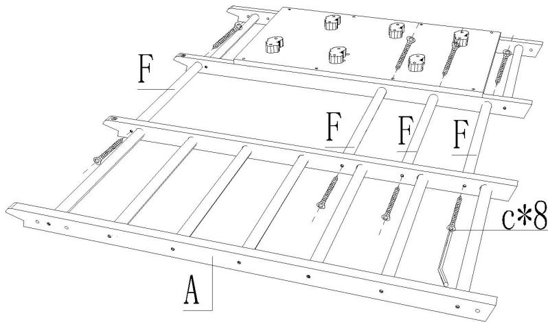
Connect 4 F round sticks between the part installed in the third step and part A, and connect with 8 pieces of M5\*35. Keep it aside for later use.
