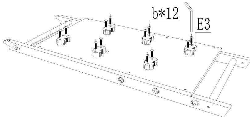
Install the climbing stone E3 on the part assembled in the second step, and then fix it with 12 pieces of **M8\*35**.
