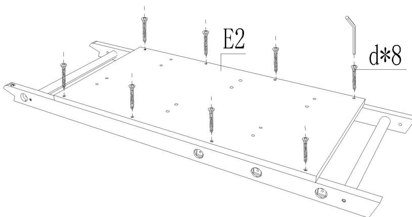
Connect board E2 to the part assembled in the first step and fix it with 8 pieces of M5\*35 screws.
