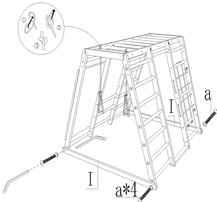
Use 4 pieces of M6\*35 screws to fix the two beams I to the bottom of the climbing frame.
